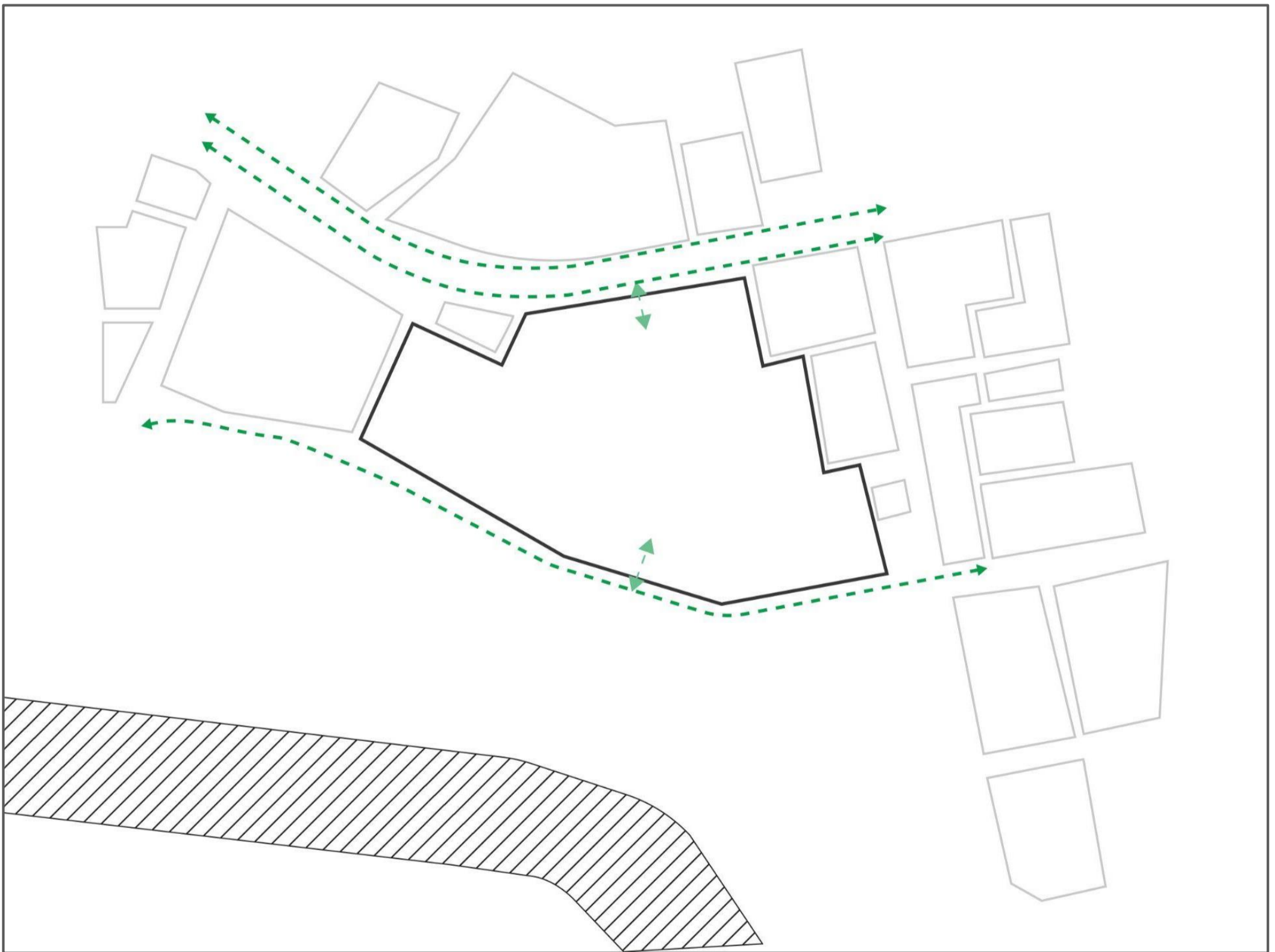
Diagram of the existing bus lane and connection to the projected site.
